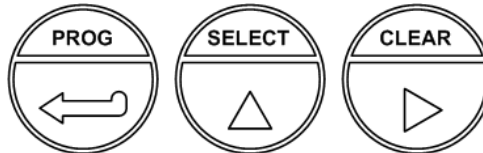
Fig. 2: Control panel, optical keys.
