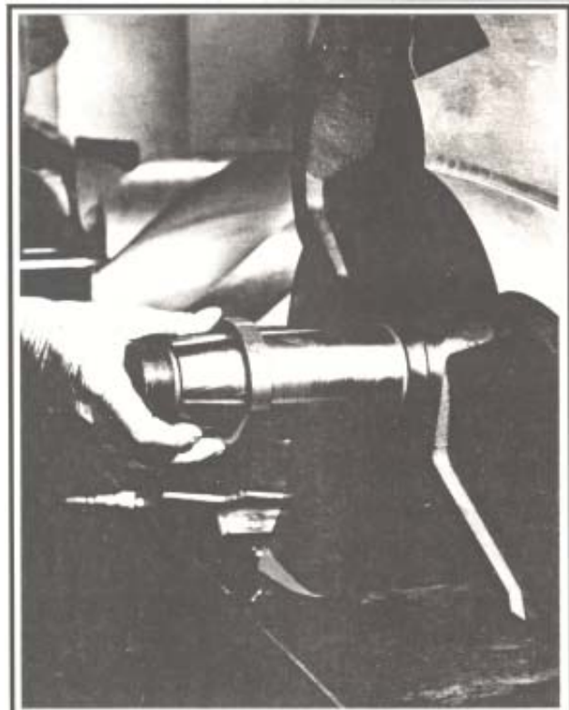
Figure 4.7 Install Ring of the Crane Seal
