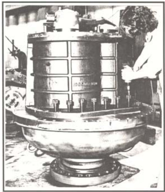
Figure 4.17 Secure All Nuts to Their Proper Torque and Mount Accessories as Desired
