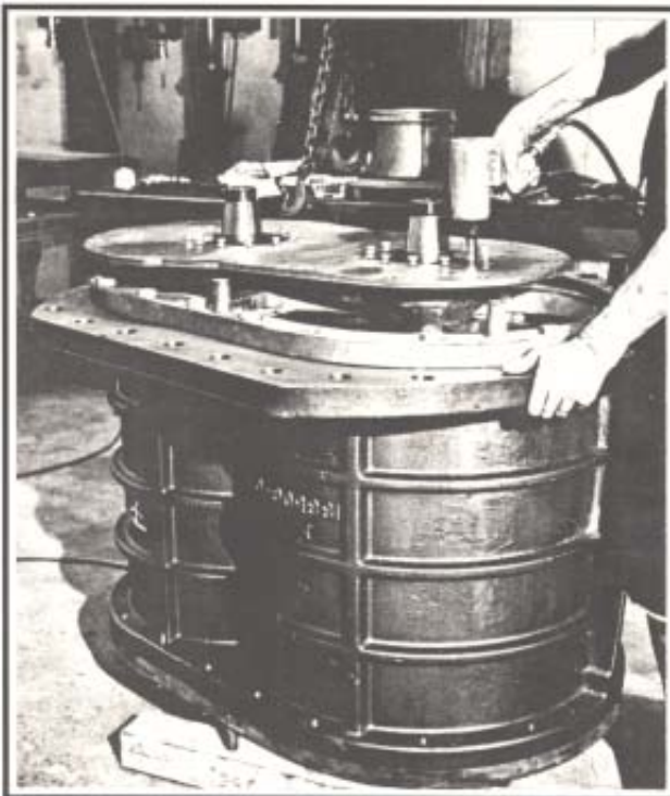
Figure 4.12 Replace Mounting Plate and Screws. The Wide End of Mounting Plate Fits Over the 4T Rotor Shaft.
