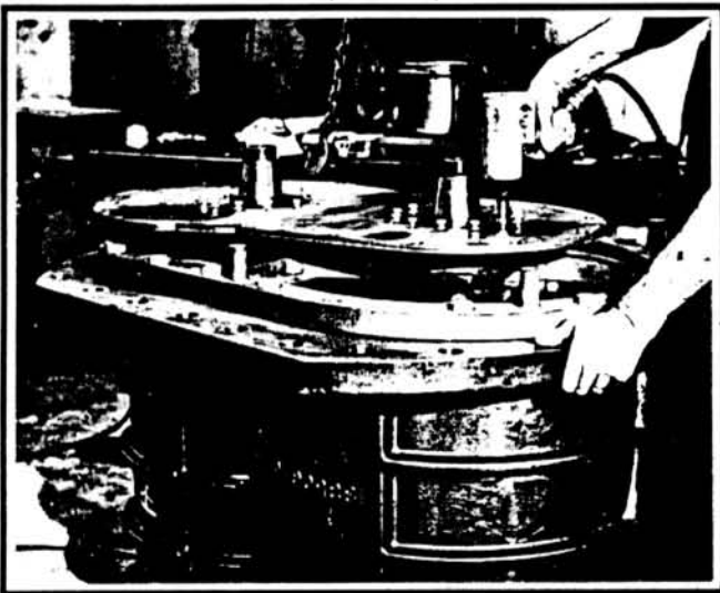
Figure 4-10 Replace mounting plate and screws. The wide end of the mounting plate fits over the four tooth
