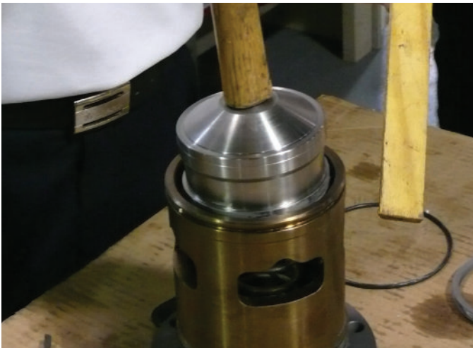
Figure 9-7 Removing Spring From Cylinder
