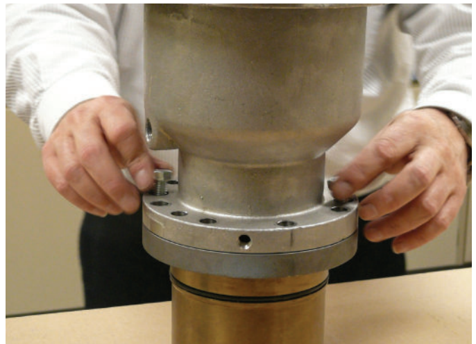
Figure 9-32 Install Motor Housing
