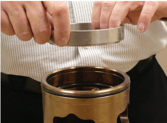
Figure 9-26 Install Seal Ring
