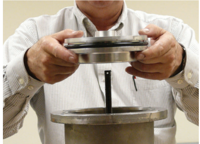
Figure 9-14 Remove Piston from Power Cylinder Assembly
