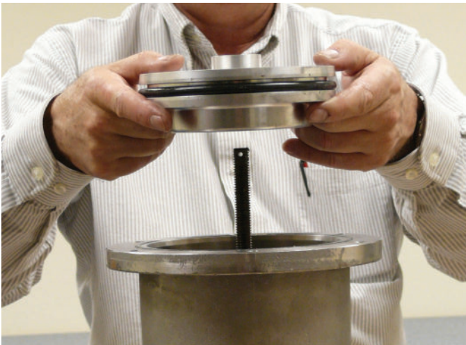
Figure 9-34 Install Motor Piston over Shaft
