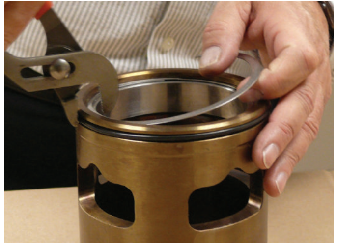
Figure 9-27 Install Retaining Ring
