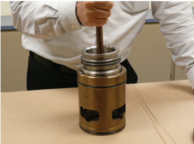
Figure 9-16 Remove Piston and Shaft Assembly
