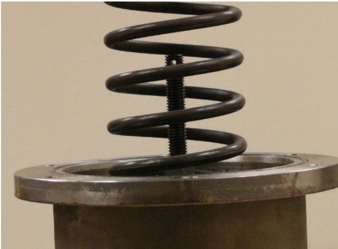
Figure 9-36 Install Spring in Housing
