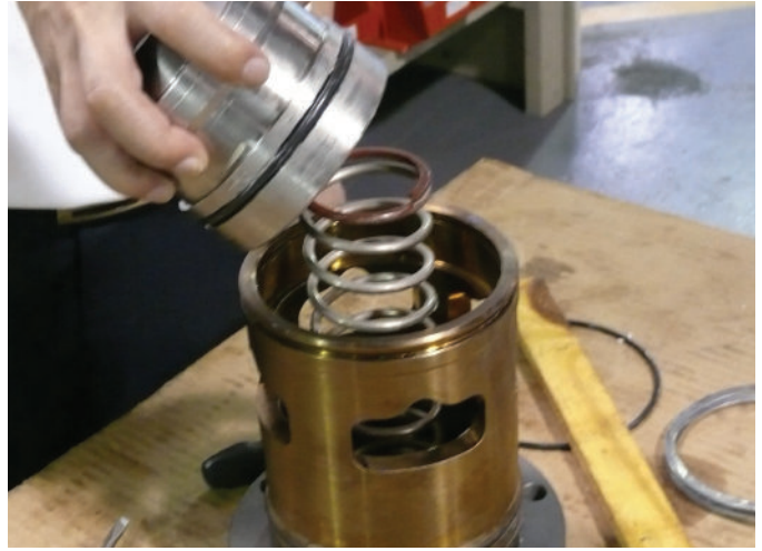
Figure 9-8 Removing Spring From Cylinder
